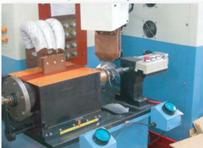
Rotor impeller spot welding
